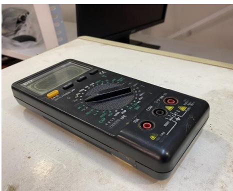
A photograph of a black digital multimeter resting on a light-colored surface. The device has a digital display and multiple buttons and ports for testing electrical signals.                   |            |
